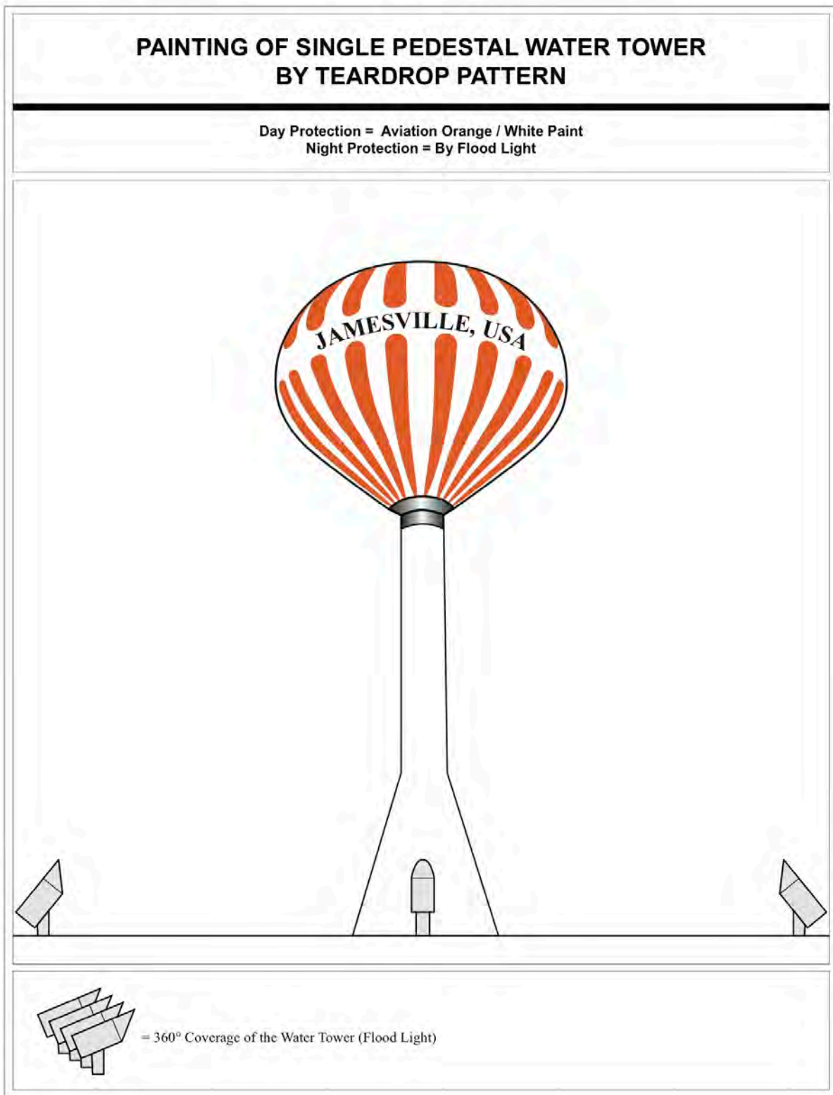
Figure A-17. Painting a Single Pedestal Water Tower Using the Teardrop Pattern
